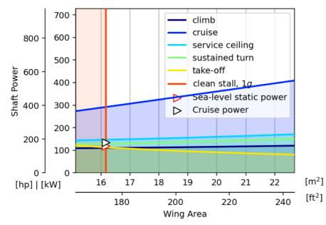
From the diagram shown, it is clear that the cruise constraint is far above the other constraints, so my be incorrect. This may be due to a high coefficient of drag.
