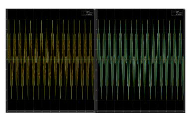
Pure P control better rejects the noise, which is good for most applications. The derivative control amplifies the noise.
