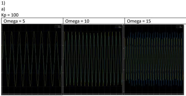
The difference between the peaks is minimised at omega = 10 and this is because this is the natural frequency of the plant
