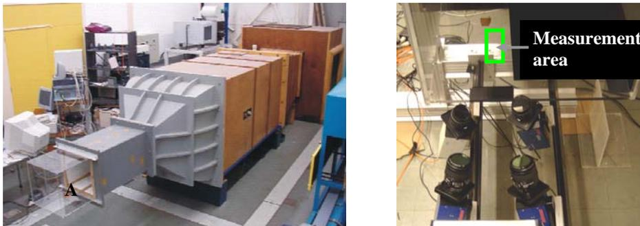
Figure 8.1. Experimental arrangement. Left: low speed wind tunnel with Plexiglas test section (A). Right: camera setup for tomographic-PIV underneath the test section (used for configurations I and II).
