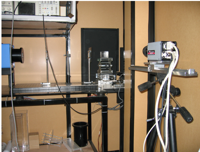
Figure 2.3: Picture of the experimental arrangement for the uniform flow simulation. Shown sitting on the traverse system is the platform jack on which sits the uniform flow block. The block contains seeding particles suspended-frozen inside it.
