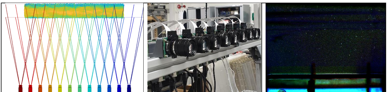
Figure 2: Illustration of planar camera array concept: (a) simulated reconstruction of 1.1 \times 10^5 particle tracks in a turbulent channel flow (b) 8-camera array installed in channel flow facility and (c) inverted shadowgraph image of particles obtained using pulsed LED backlighting. Initial tests show that sharp particle images can be obtained with good depth of field for volumetric PTV.
