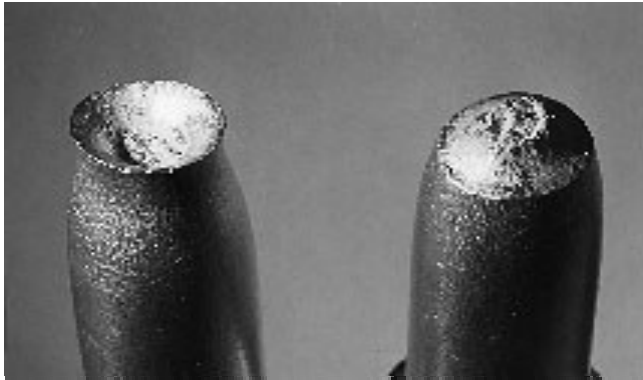
Typical cup-cone failure: tensile test
