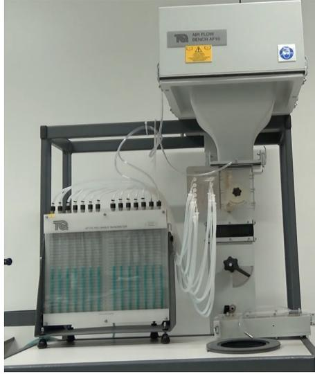
Figure 1: Air flow bench with manometer shown
